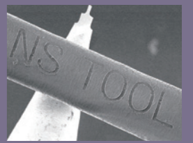
With "Micro Edge" with cutting edge diameter 0.01 mm, we engraved the letters "NS TOOL" on hair.
